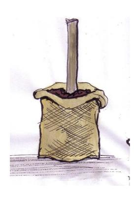
Make sure the soil is slightly compacted to allow the sack to stand straight up.
