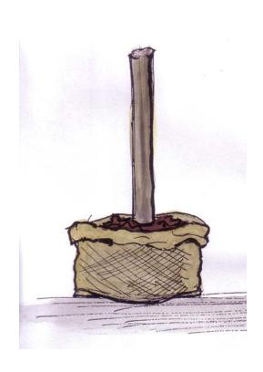
Place a sack on the ground. Place a 4 inch diameter post in the middle of the sack. Start filling a mixture of 2/3 topsoil and 1/3 compost around the post – pack this mixture and keep filling.
